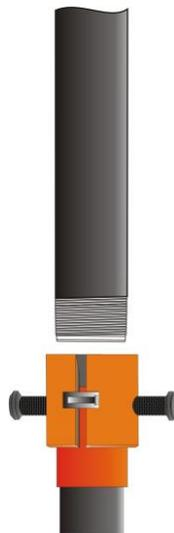
**Figure 5 – Make-up with special bell guide**
