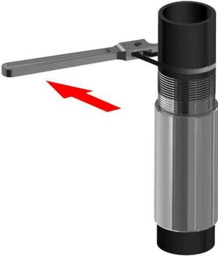
**Figure 10 – Make-up start with strap tongs**
