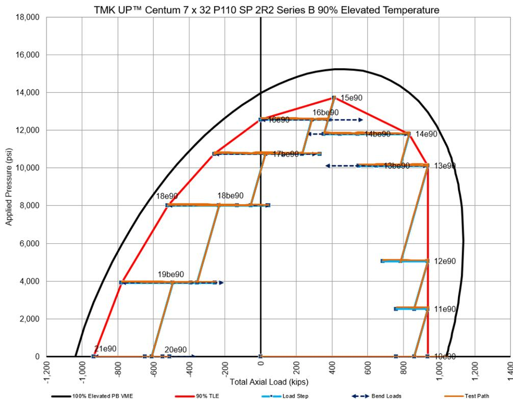
**Figure 1-19: Test Envelope for TMK UP CENTUM Specimen 2R2 Series B (90% Elevated)**
