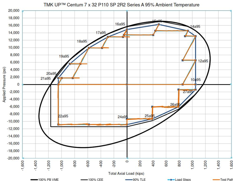
**Figure 1-26: Test Envelope for TMK UP CENTUM Specimen 2R2 Series A (95% Ambient)**
