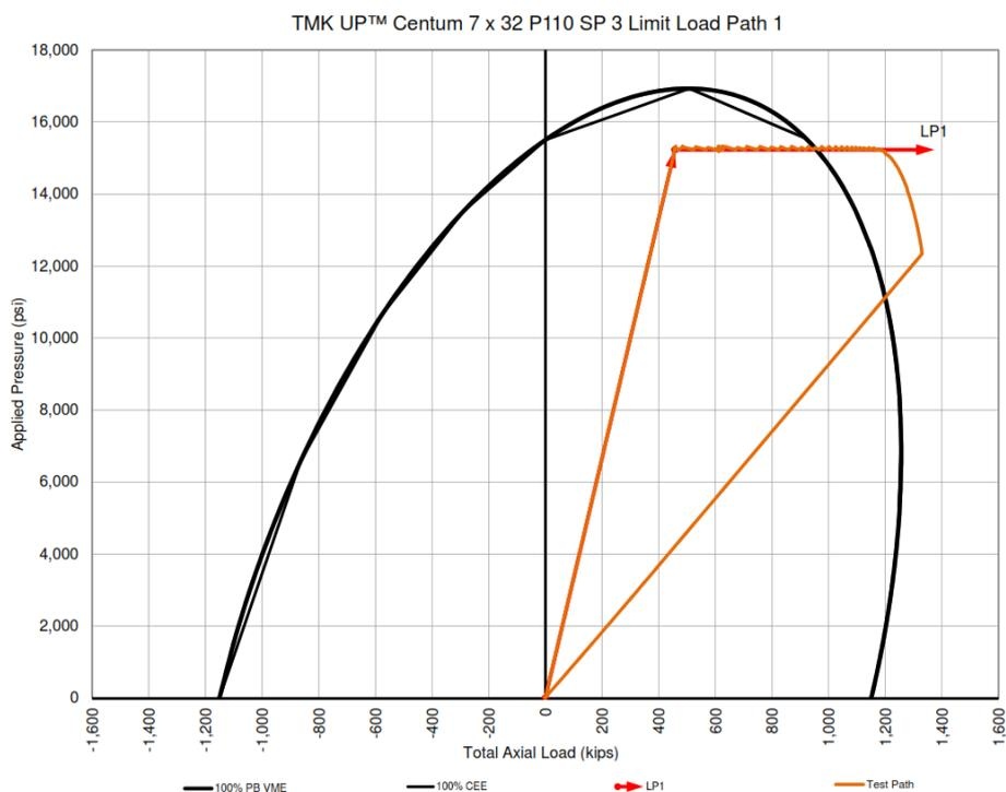
**Figure 1-38:** Limit Load Path 1 for TMK UP CENTUM Specimen 3
