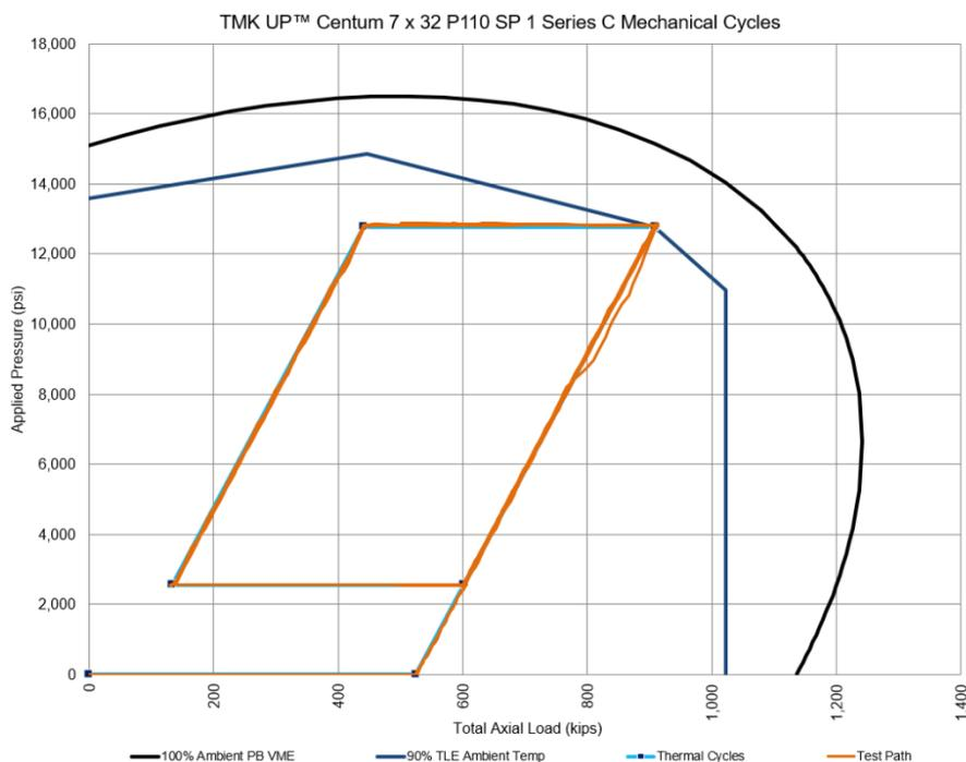
**Figure 1-7: Test Envelope for TMK UP CENTUM Specimen 1 Series C Mechanical Cycles**
