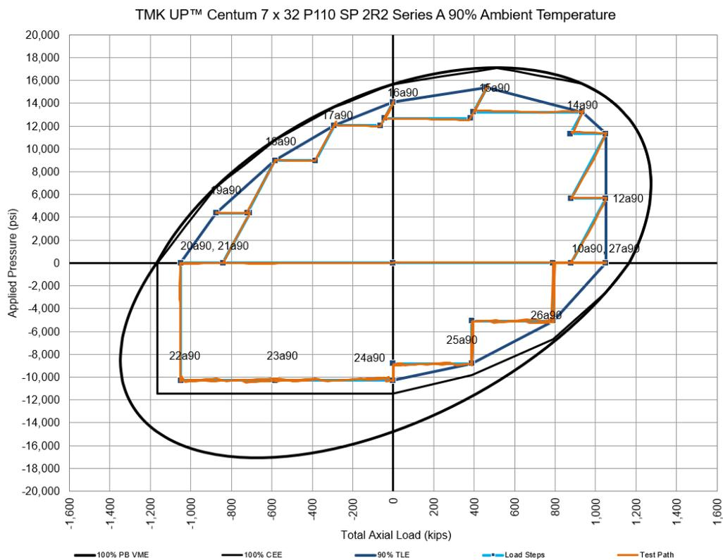
**Figure 1-25: Test Envelope for TMK UP CENTUM Specimen 2R2 Series A (90% Ambient)**
