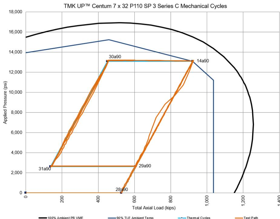
**Figure 1-33: Test Envelope for TMK UP CENTUM Specimen 3 Series C Mechanical Cycles**
