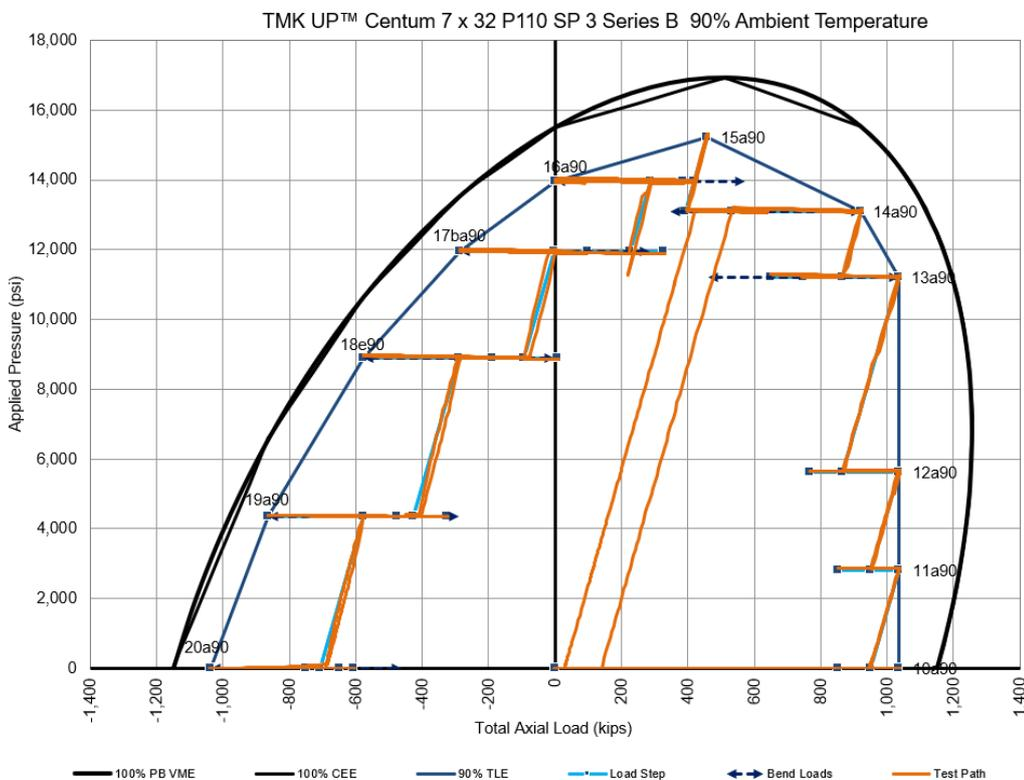
**Figure 1-31: Test Envelope for TMK UP CENTUM Specimen 3 Series B (90% Ambient)**
