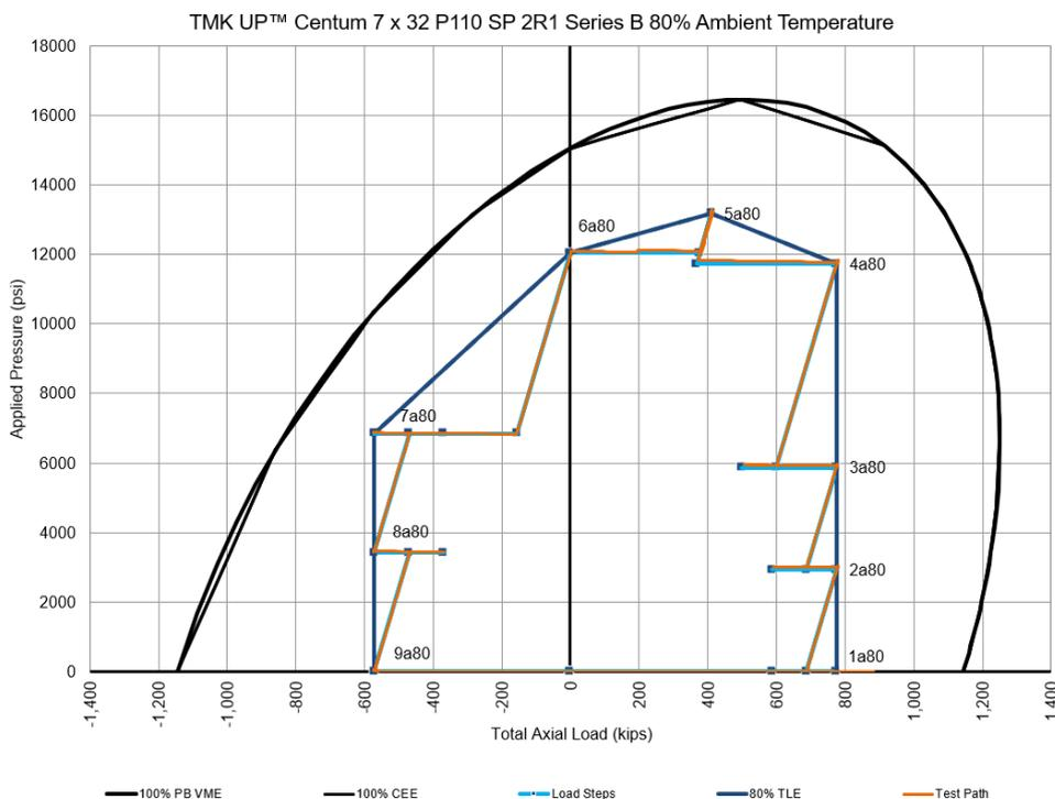
**Figure 1-15: Test Envelope for TMK UP CENTUM Specimen 2R1 Series B (80% Ambient)**
