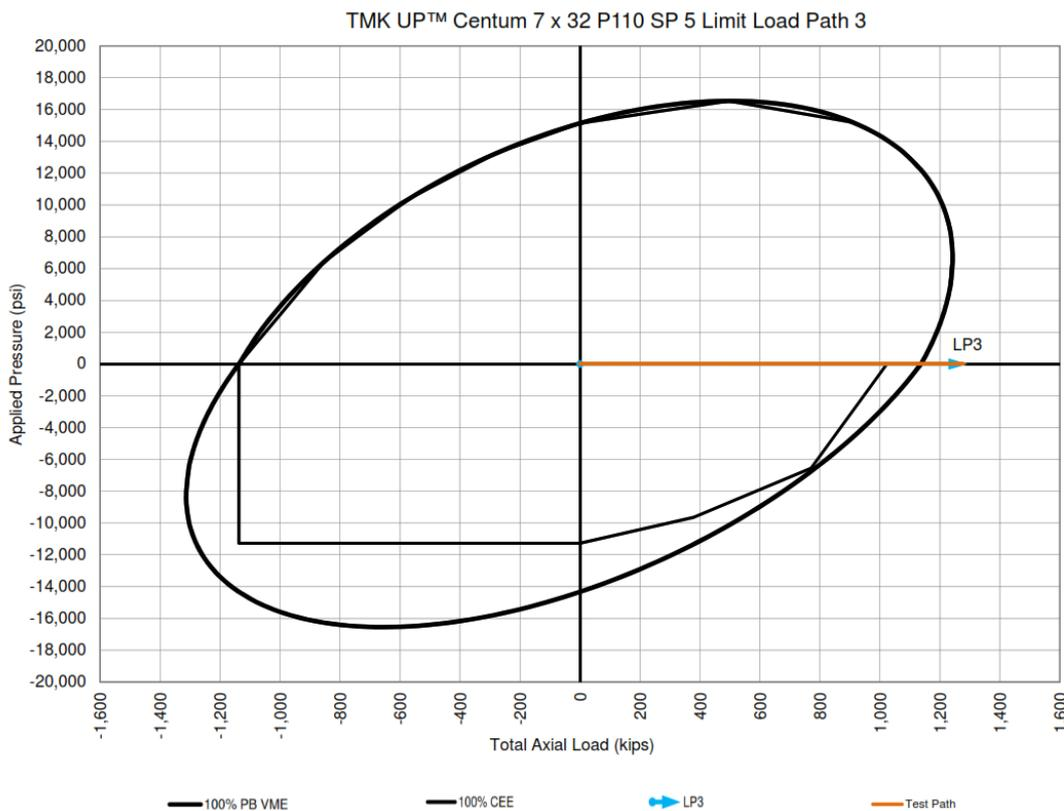
**Figure 1-50:** Limit Load Path for TMK UP CENTUM Specimen 5
