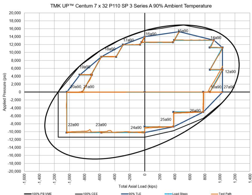
**Figure 1-36: Test Envelope for TMK UP CENTUM Specimen 3 Series A (90% Ambient)**
