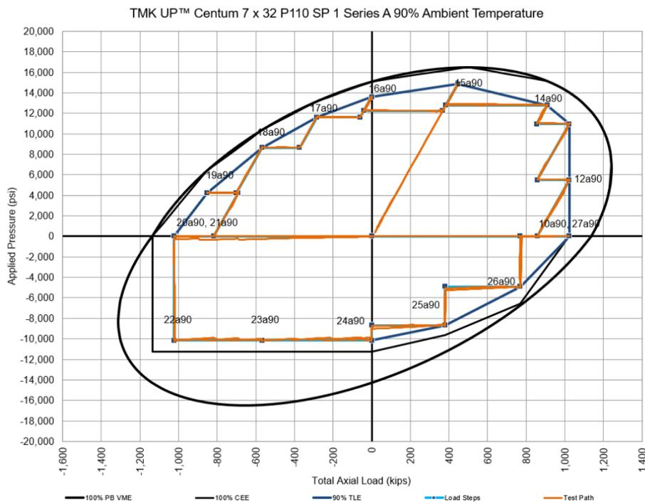
**Figure 1-10: Test Envelope for TMK UP CENTUM Specimen 1 Series A (90% Ambient)**
