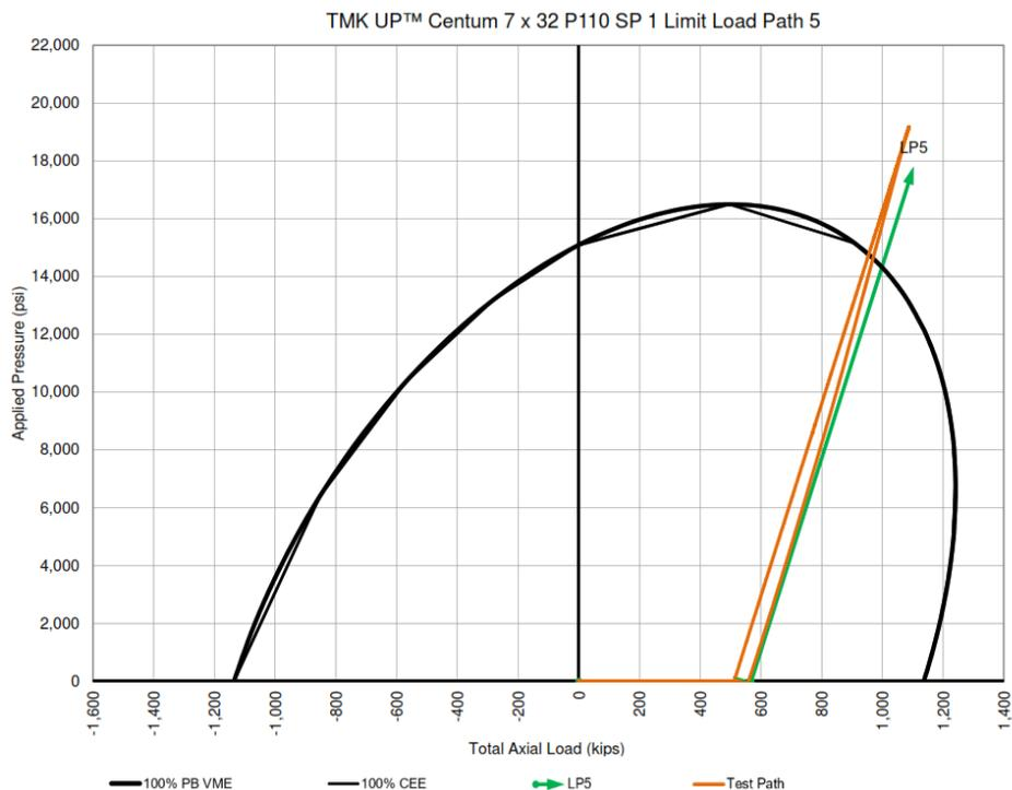
**Figure 1-12: Limit Load Path for TMK UP CENTUM Specimen 1**
