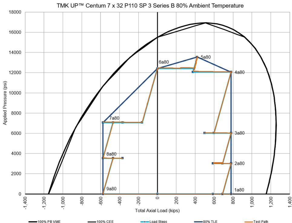
**Figure 1-28: Test Envelope for TMK UP CENTUM Specimen 3 Series B (80% Ambient)**
