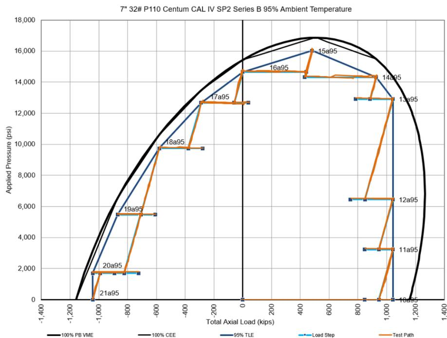
**Figure 1-14: Test Envelope for TMK UP CENTUM Specimen 2 Series B (95% Ambient)**
