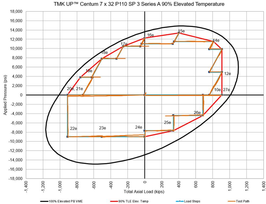
**Figure 1-34: Test Envelope for TMK UP CENTUM Specimen 3 Series A (90% Elevated)**
