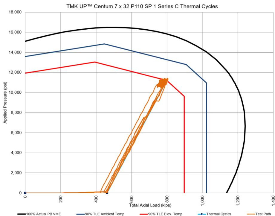
**Figure 1-6: Test Envelope for TMK UP CENTUM Specimen 1 Series C Thermal Cycles**
