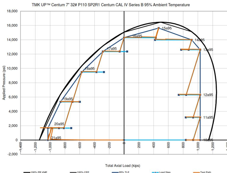
**Figure 1-53: Specimen 2R1 Series B 95% Test Path**
