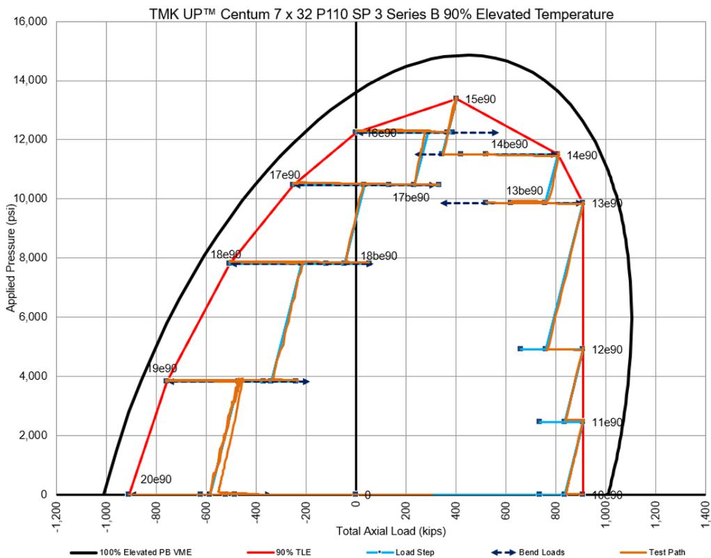
**Figure 1-30: Test Envelope for TMK UP CENTUM Specimen 3 Series B (90% Elevated)**
