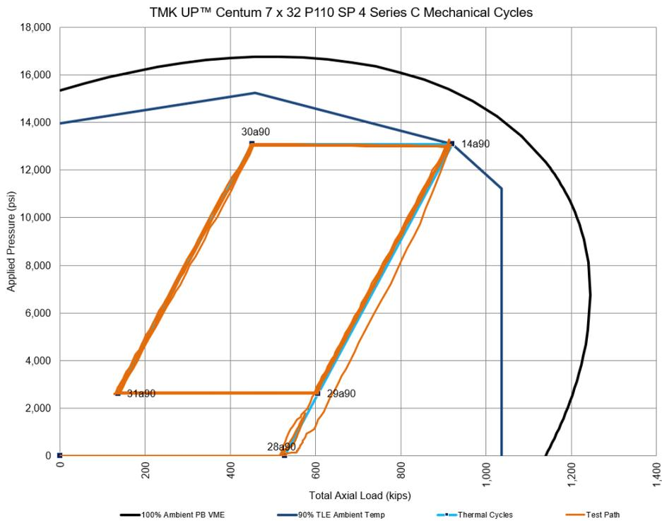
**Figure 1-44: Test Envelope for TMK UP CENTUM Specimen 4 Series C Mechanical Cycles**
