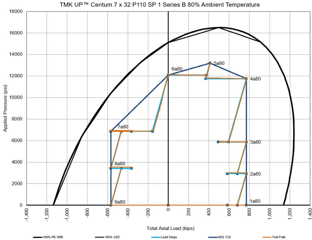
**Figure 1-2: Test Envelope for TMK UP CENTUM Specimen 1 Series B (80% Ambient)**
