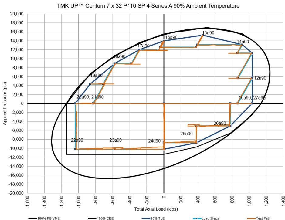
**Figure 1-47: Test Envelope for TMK UP CENTUM Specimen 4 Series A (90% Ambient)**
