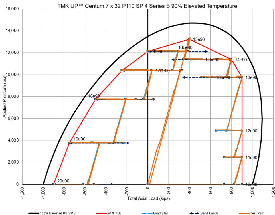
**Figure 1-41: Test Envelope for TMK UP CENTUM Specimen 4 Series B (90% Elevated)**
