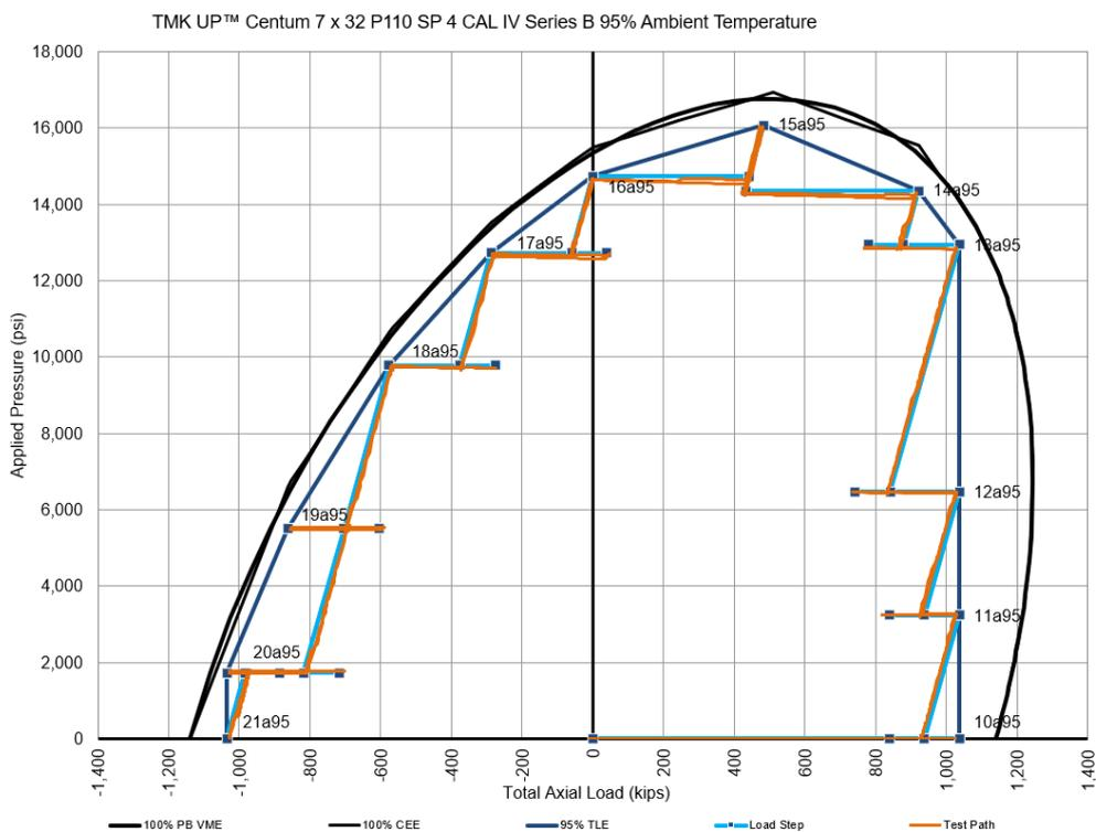
**Figure 1-40: Test Envelope for TMK UP CENTUM Specimen 4 Series B (95% Ambient)**
