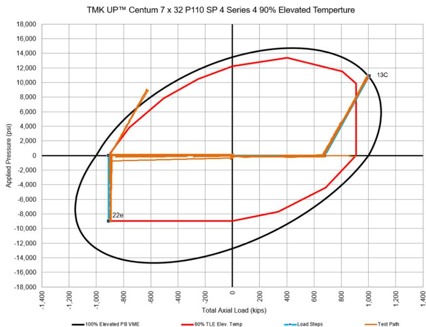
**Figure 1-46: Test Envelope for TMK UP CENTUM Specimen 4 Series A QI-QIII Cycles**
