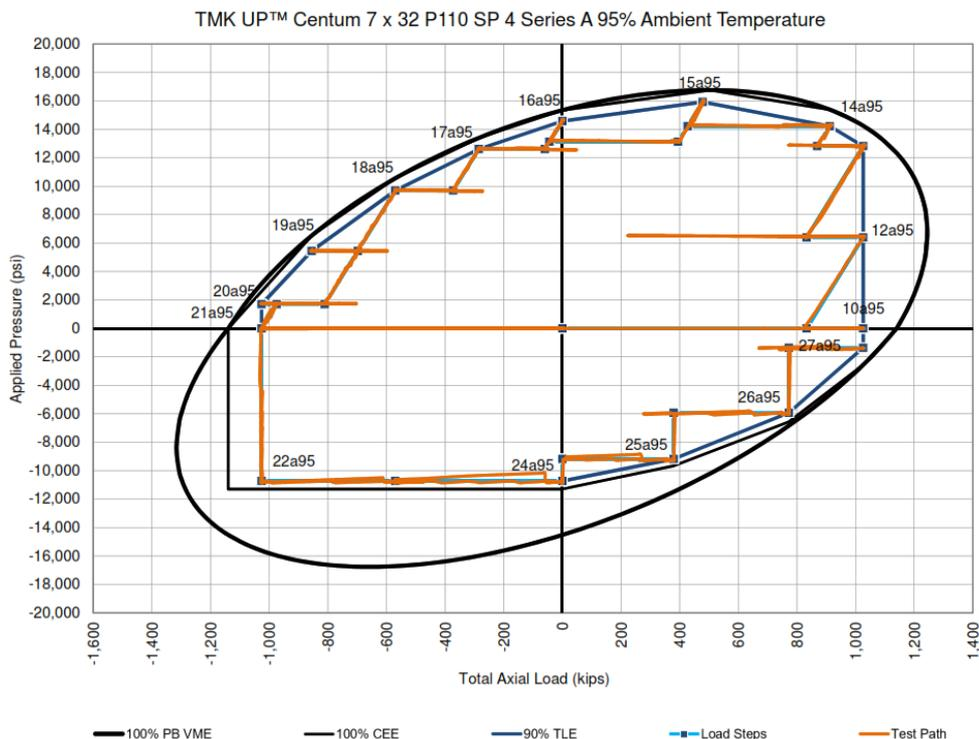
**Figure 1-48: Test Envelope for TMK UP CENTUM Specimen 4 Series A (95% Ambient)**
