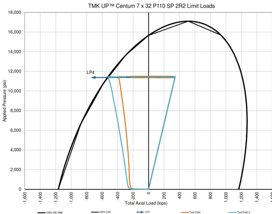
**Figure 1-27:** Limit Load Path for TMK UP CENTUM Specimen 2R2
