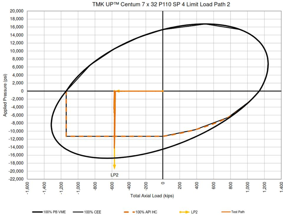
**Figure 1-49: Limit Load Path for TMK UP CENTUM Specimen 4**
