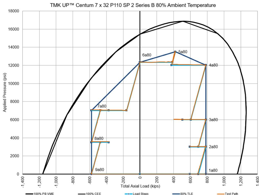
**Figure 1-13: Test Envelope for TMK UP CENTUM Specimen 2 Series B (80% Ambient)**
