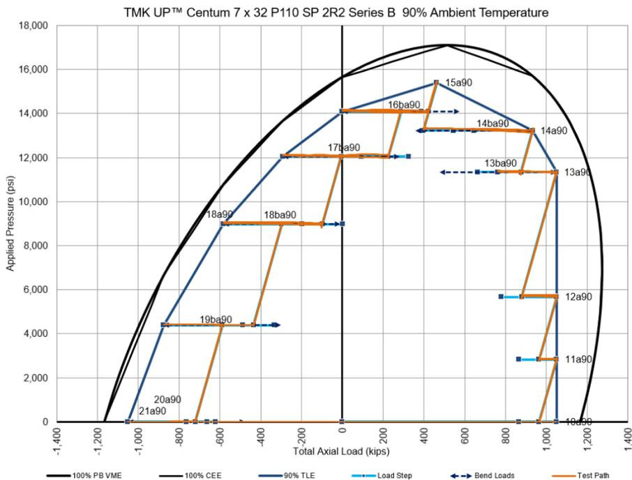
**Figure 1-20: Test Envelope for TMK UP CENTUM Specimen 2R2 Series B (90% Ambient)**
