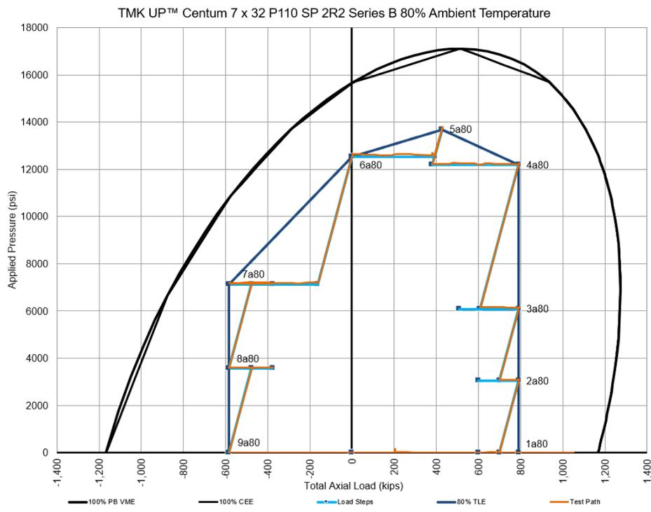
**Figure 1-17: Test Envelope for TMK UP CENTUM Specimen 2R2 Series B (80% Ambient)**
