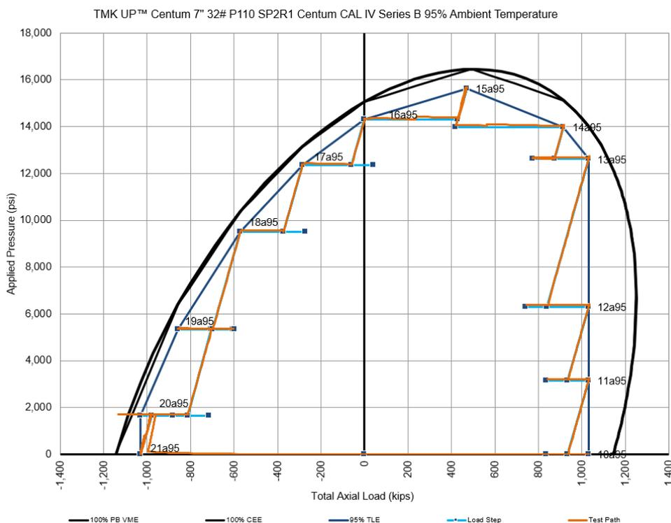
**Figure 1-16: Test Envelope for TMK UP CENTUM Specimen 2R1 Series B (95% Ambient)**
