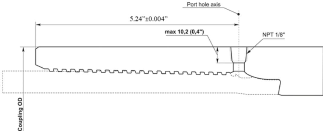
**Figure 1-1: Port Holes Location And Size**
