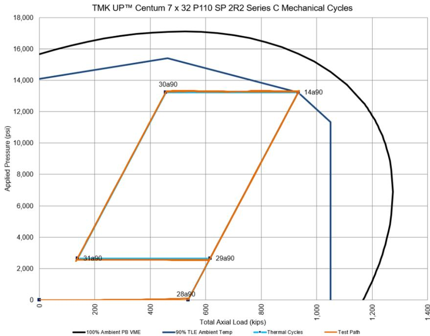
**Figure 1-22: Test Envelope for TMK UP CENTUM Specimen 2R2 Series C Mechanical Cycles**
