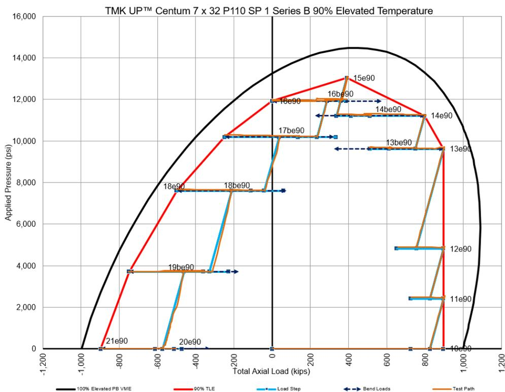
**Figure 1-4: Test Envelope for TMK UP CENTUM Specimen 1 Series B (90% Elevated)**
