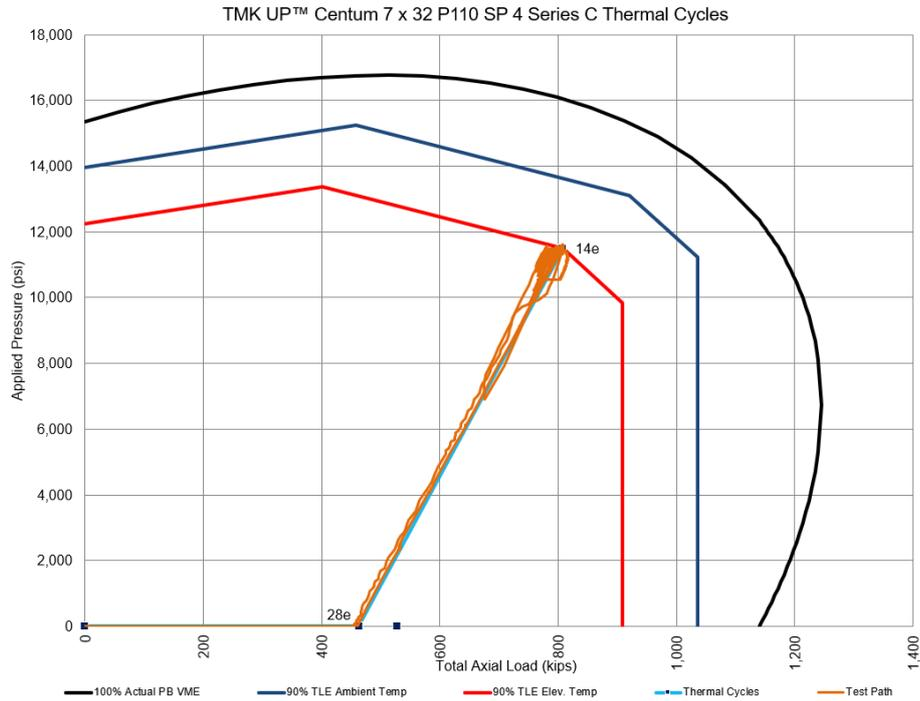
**Figure 1-43: Test Envelope for TMK UP CENTUM Specimen 4 Series C Thermal Cycles**
