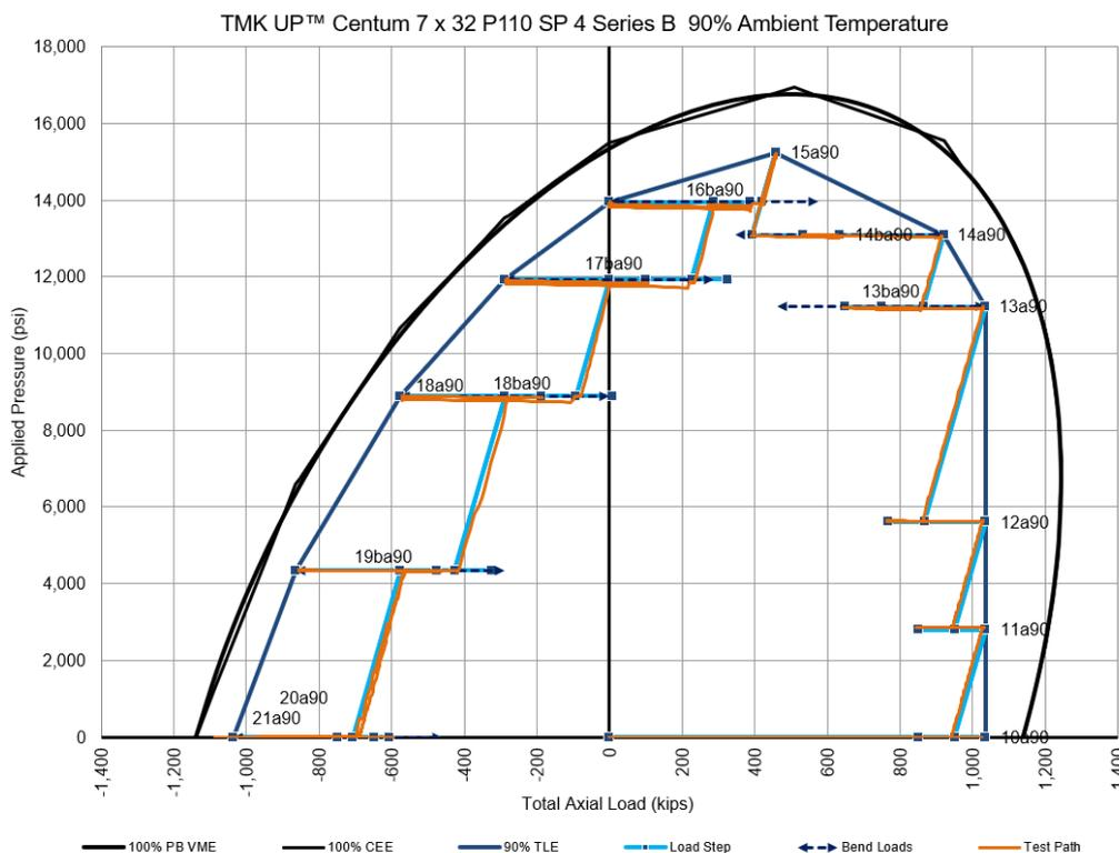
**Figure 1-42: Test Envelope for TMK UP CENTUM Specimen 4 Series B (90% Ambient)**
