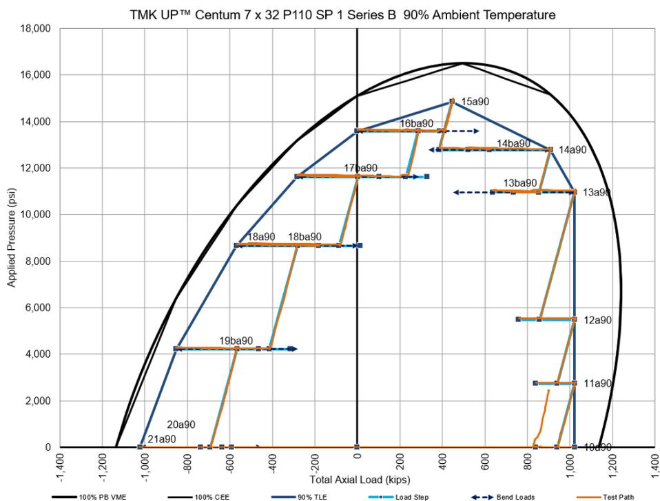
**Figure 1-5: Test Envelope for TMK UP CENTUM Specimen 1 Series B (90% Ambient)**
