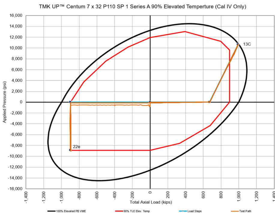
**Figure 1-9: Test Envelope for TMK UP CENTUM Specimen 1 Series A QI-QIII Cycles**
