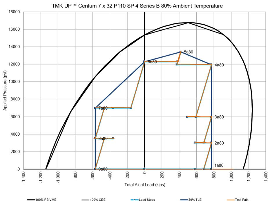
**Figure 1-39: Test Envelope for TMK UP CENTUM Specimen 4 Series B (80% Ambient)**
