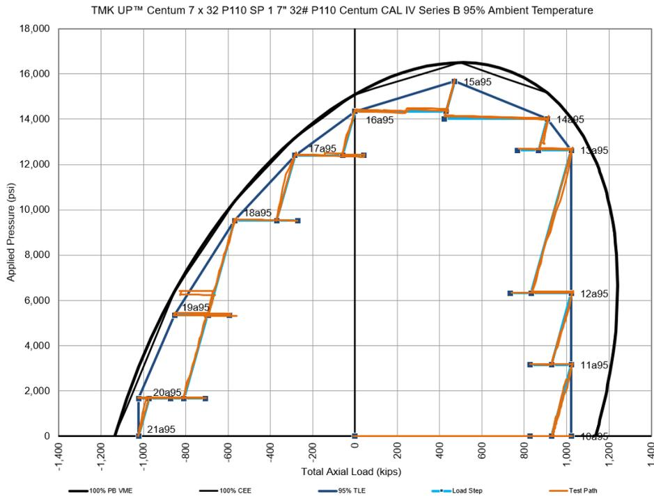
**Figure 1-3: Test Envelope for TMK UP CENTUM Specimen 1 Series B (95% Ambient)**
