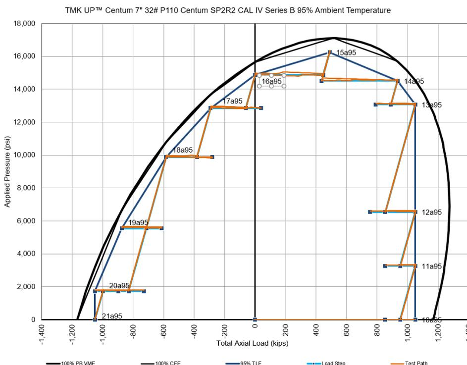
**Figure 1-18: Test Envelope for TMK UP CENTUM Specimen 2R2 Series B (95% Ambient)**
