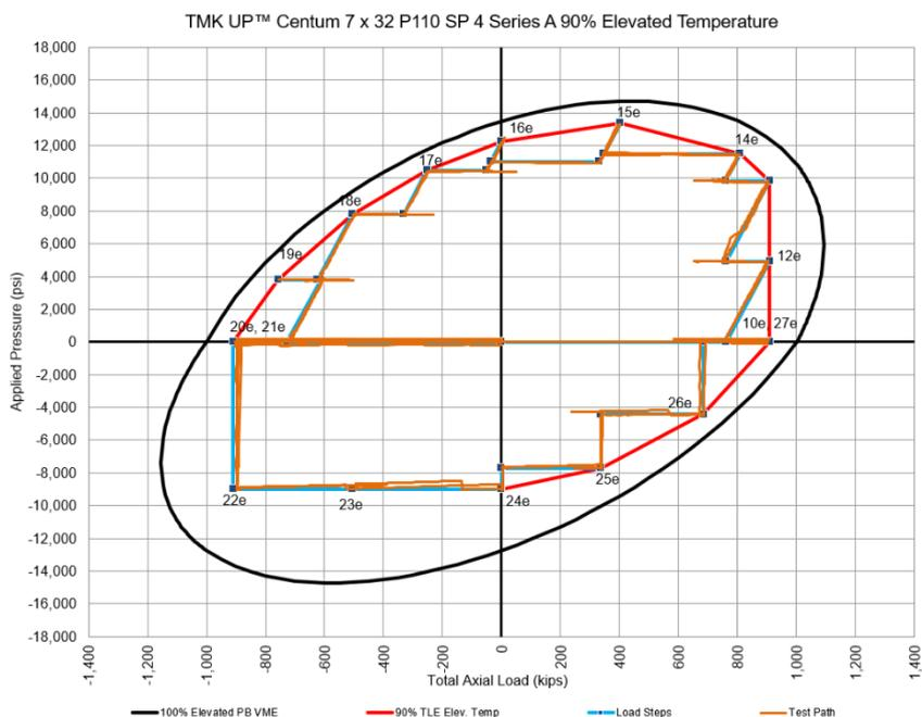
**Figure 1-45: Test Envelope for TMK UP CENTUM Specimen 4 Series A (90% Elevated)**
