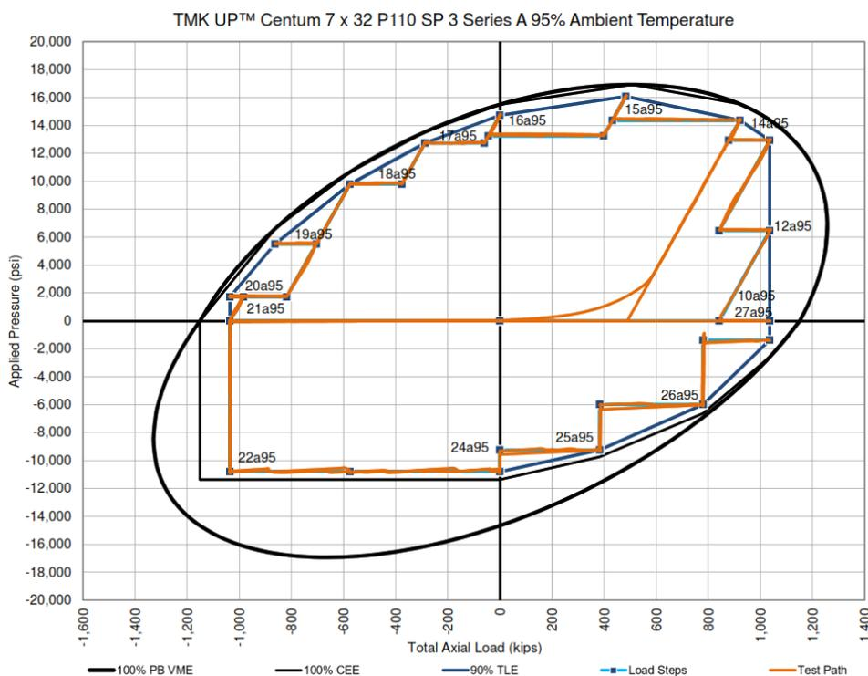
**Figure 1-37: Test Envelope for TMK UP CENTUM Specimen 3 Series A (95% Ambient)**
