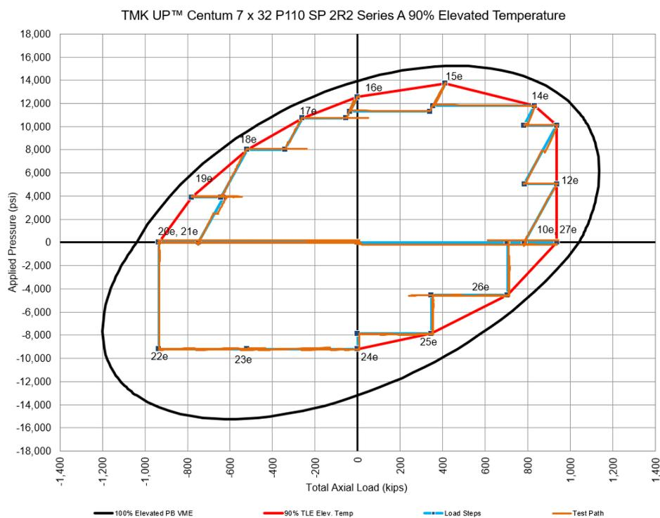
**Figure 1-23: Test Envelope for TMK UP CENTUM Specimen 2R2 Series A (90% Elevated)**
