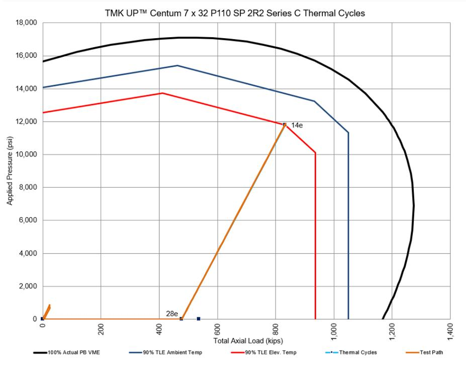
**Figure 1-21: Test Envelope for TMK UP CENTUM Specimen 2R2 Series C Thermal Cycles**
