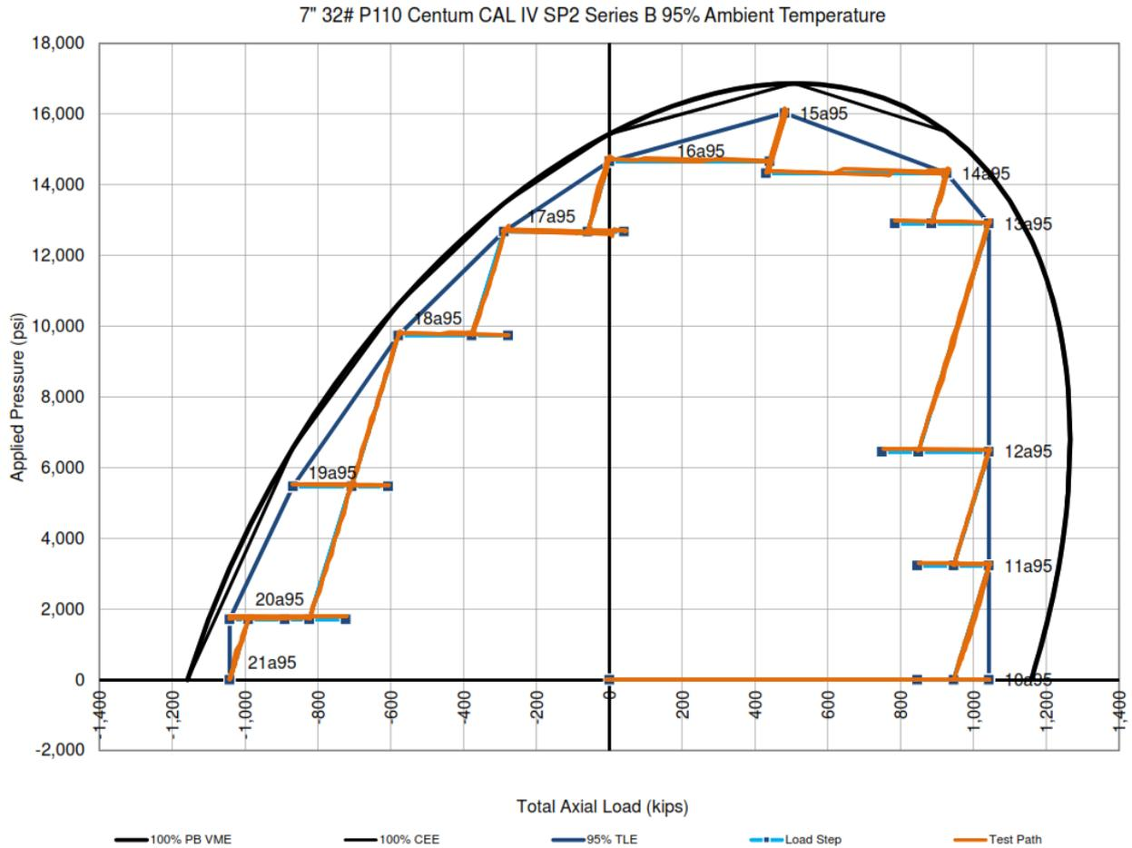
**Figure 1-51: Specimen 2 Series B 95% Test Path**
