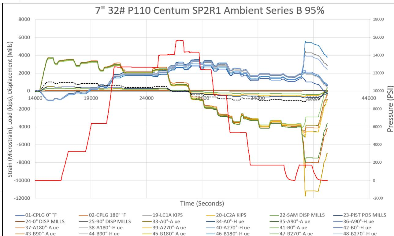
**Figure 1-54: Specimen 2R1 Series B 95% Strain Gage Data**
