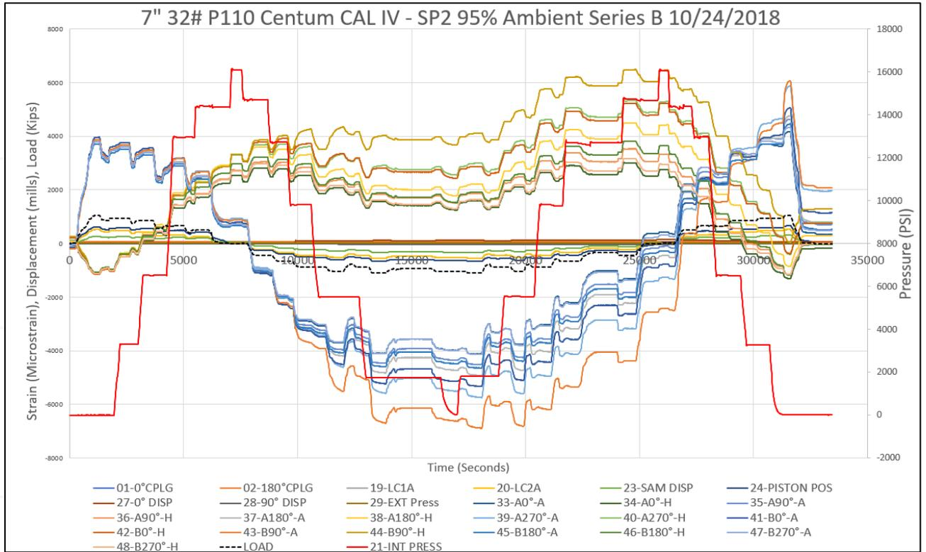
**Figure 1-52: Specimen 2 Series B Strain Gage Data**
