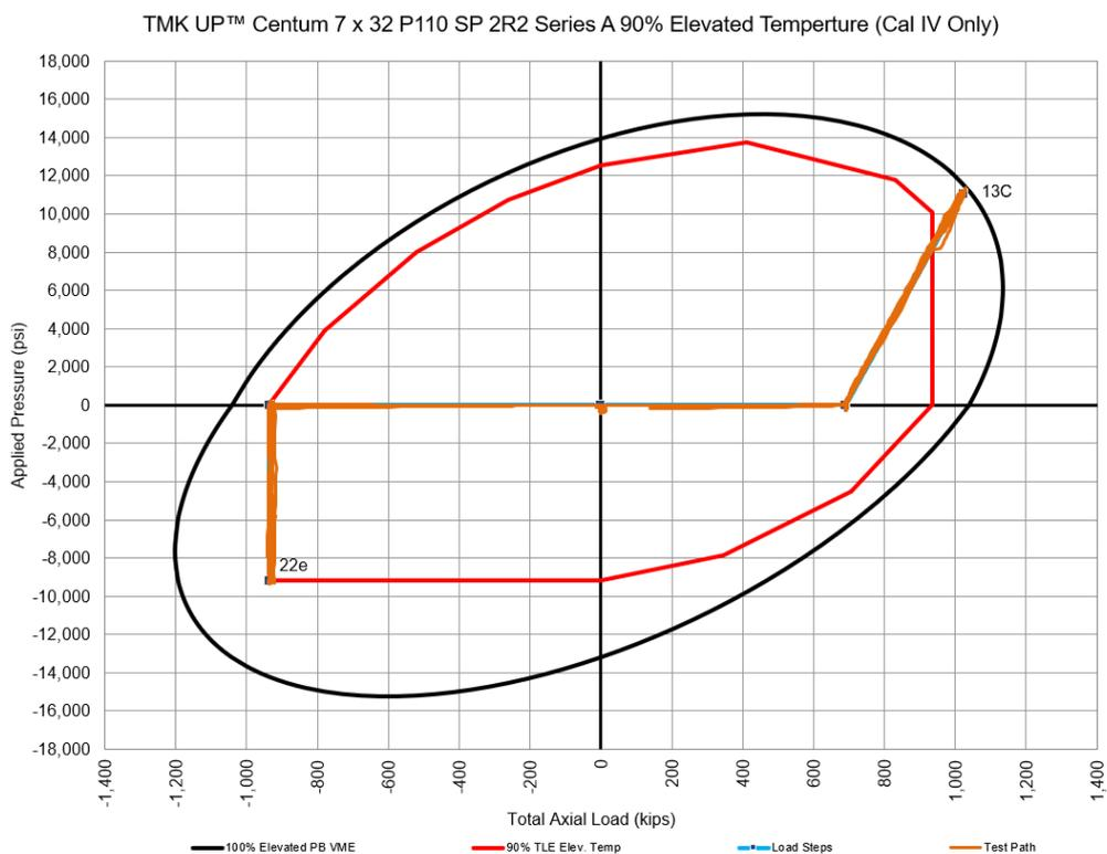
**Figure 1-24: Test Envelope for TMK UP CENTUM Specimen 2R2 Series A QI-QIII Cycles**
