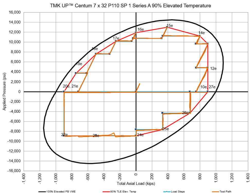
**Figure 1-8: Test Envelope for TMK UP CENTUM Specimen 1 Series A (90% Elevated)**
