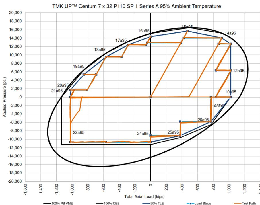
**Figure 1-11: Test Envelope for TMK UP CENTUM Specimen 1 Series A (95% Ambient)**
