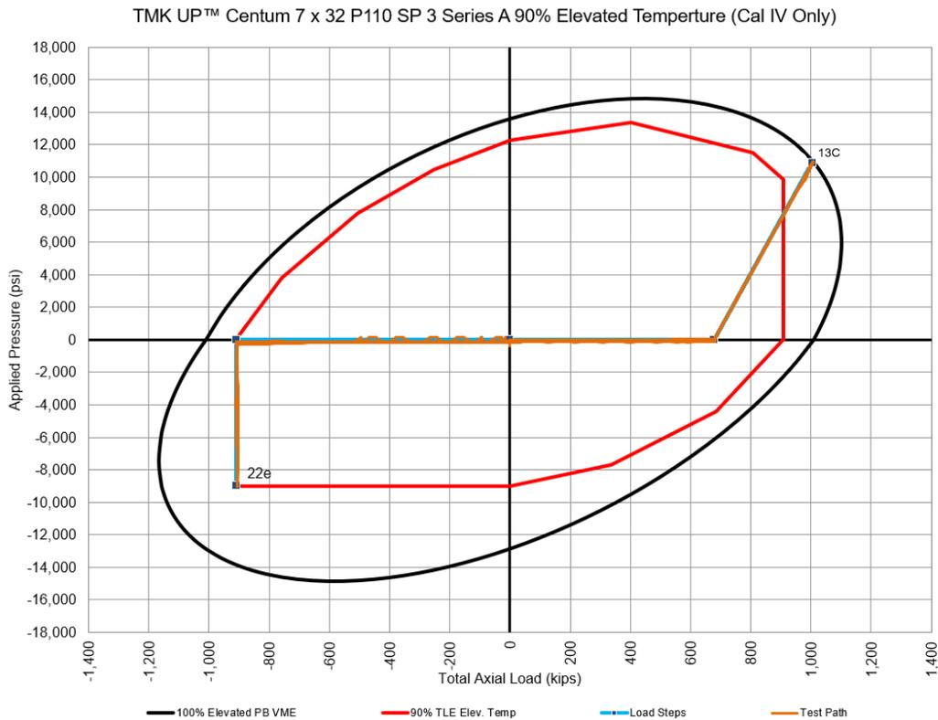
**Figure 1-35: Test Envelope for TMK UP CENTUM Specimen 3 Series A QI-QIII Cycles**
