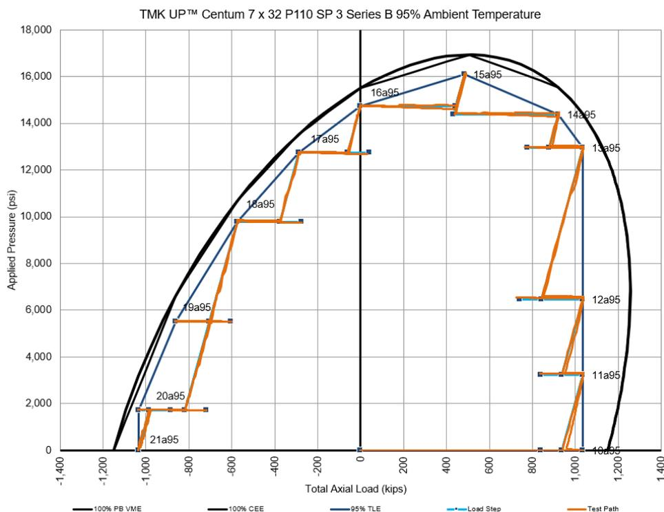
**Figure 1-29: Test Envelope for TMK UP CENTUM Specimen 3 Series B (95% Ambient)**
