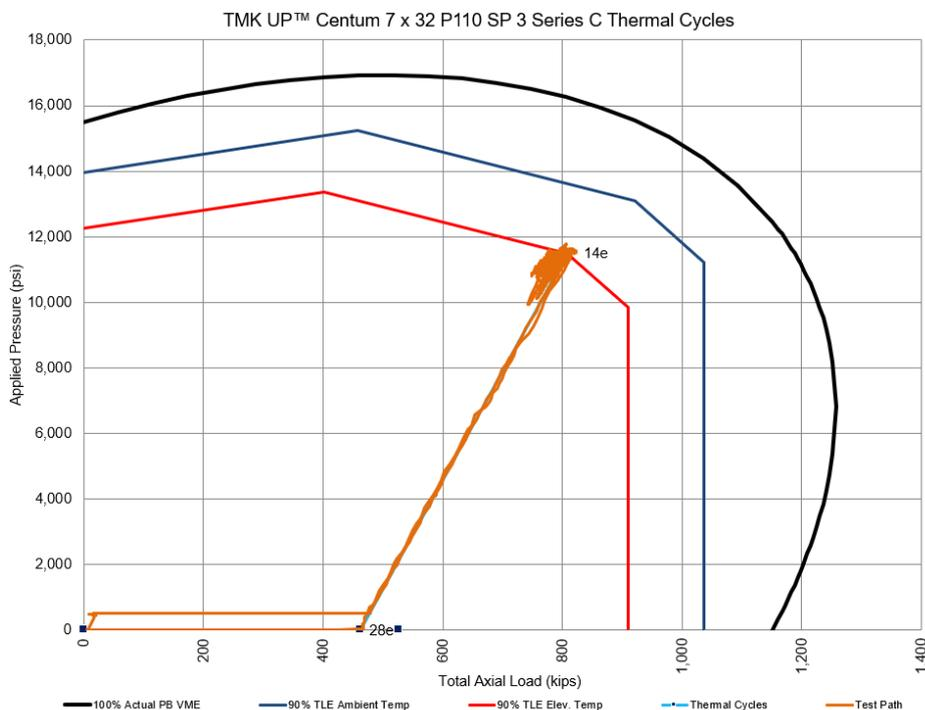
**Figure 1-32: Test Envelope for TMK UP CENTUM Specimen 3 Series C Thermal Cycles**
